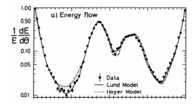
In a three-jet event there are more energy between the g and  $g - \bar{q}$  jets than between  $q - \bar{q}$ .
