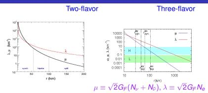
Regions of synchronized oscillations, bipolar oscillations, spectral split and MSW effects are well-separated.
