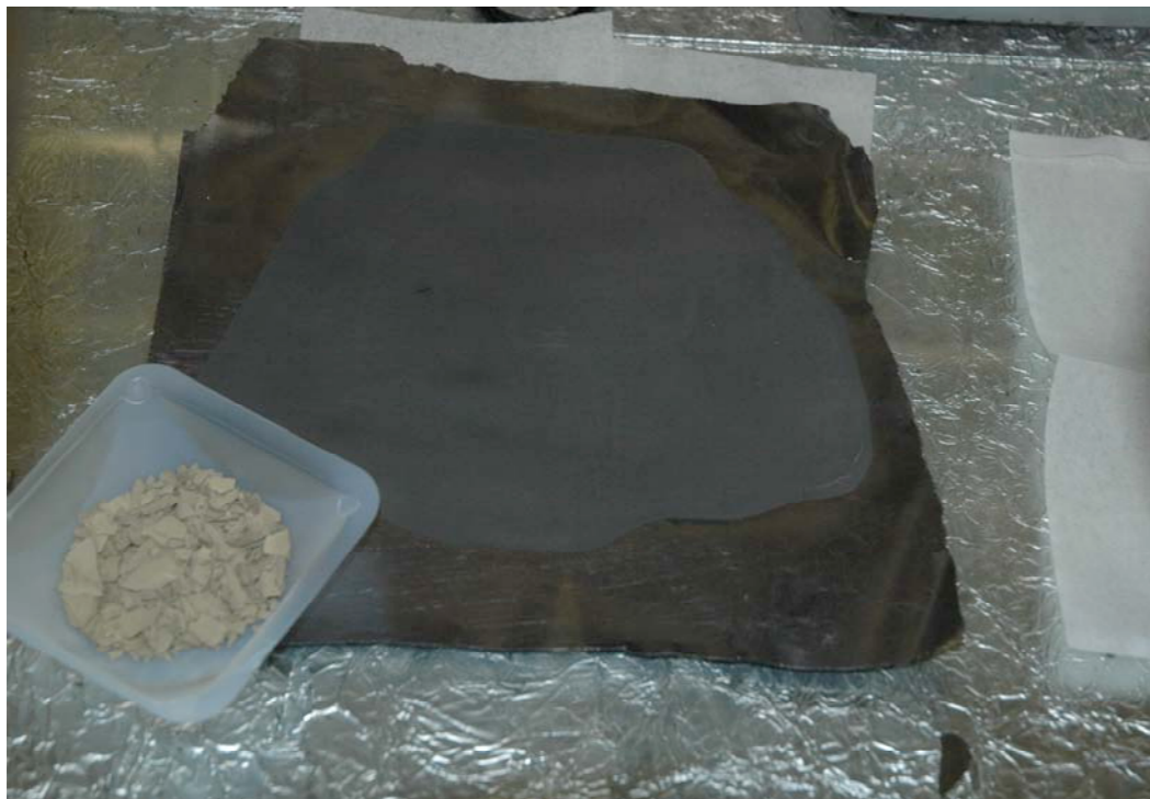
Slip cast onto exfoliated graphite foil (0.13 mm thick)
