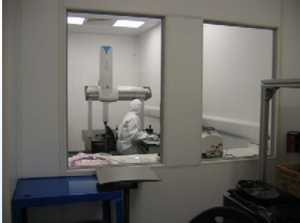
Class 1000 cleanroom with large ultra-clean laminar flow cabinet for bonding operations
