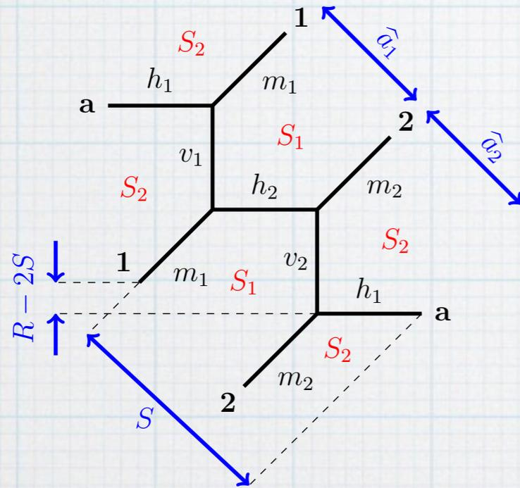
$$\begin{aligned} \hat{a}_1 &= v_1 + h_2, & \hat{a}_2 &= v_2 + h_1, \\ S &= h_2 + v_2 + h_1, & R - 2S &= m_1 - v_2. \end{aligned}$$
