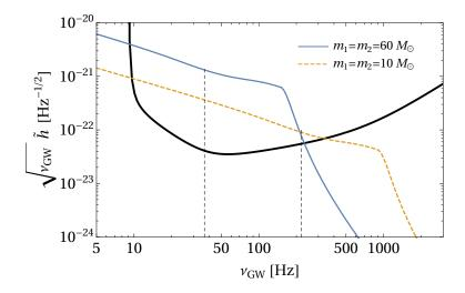
Let's consider the noise curve of the interferometer. The coalescence signal looks like the curves in the figure, with an amplitude which change smoothly as the frequency increases, has a small bump at merger, and then rapidly drops down. Roughly speaking, the maximim frequency is that of the last stable orbit, after which there is the coalescence; typically, the maximim frequency scales (like all frequencies involved in BH systems) as the inverse of the mass.
