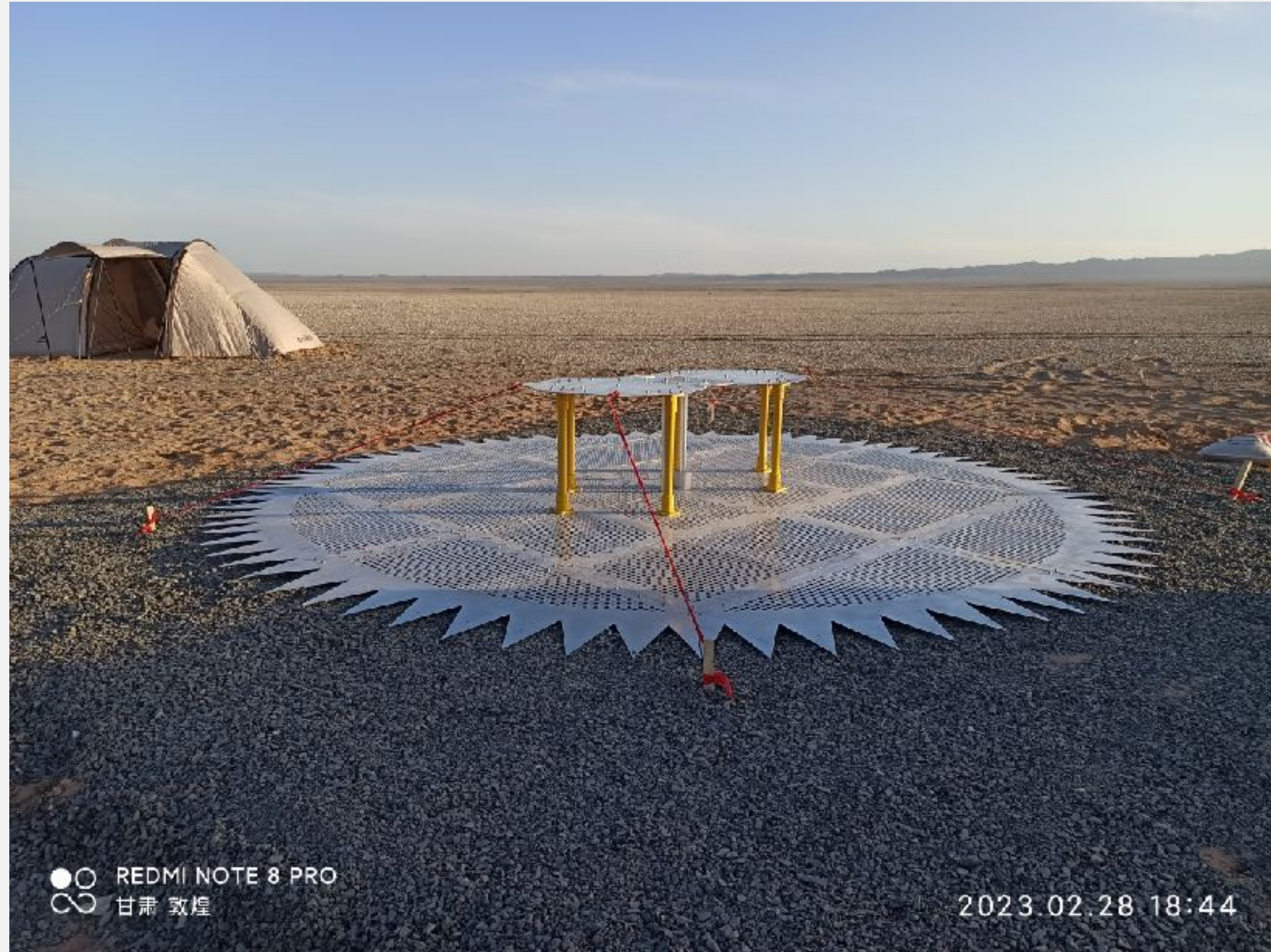
First type of Antennas available Low frequency 50 – 200 Mhz
