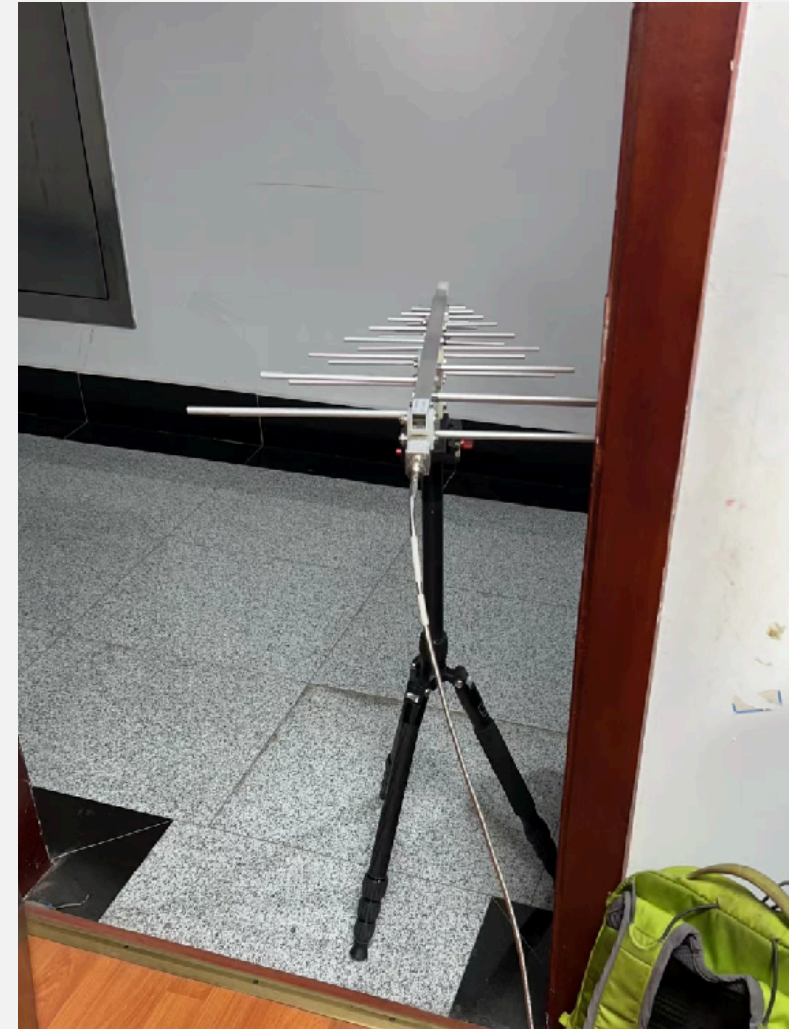
Second type of Antennas available Low frequency 0.3 – 3 Ghz
