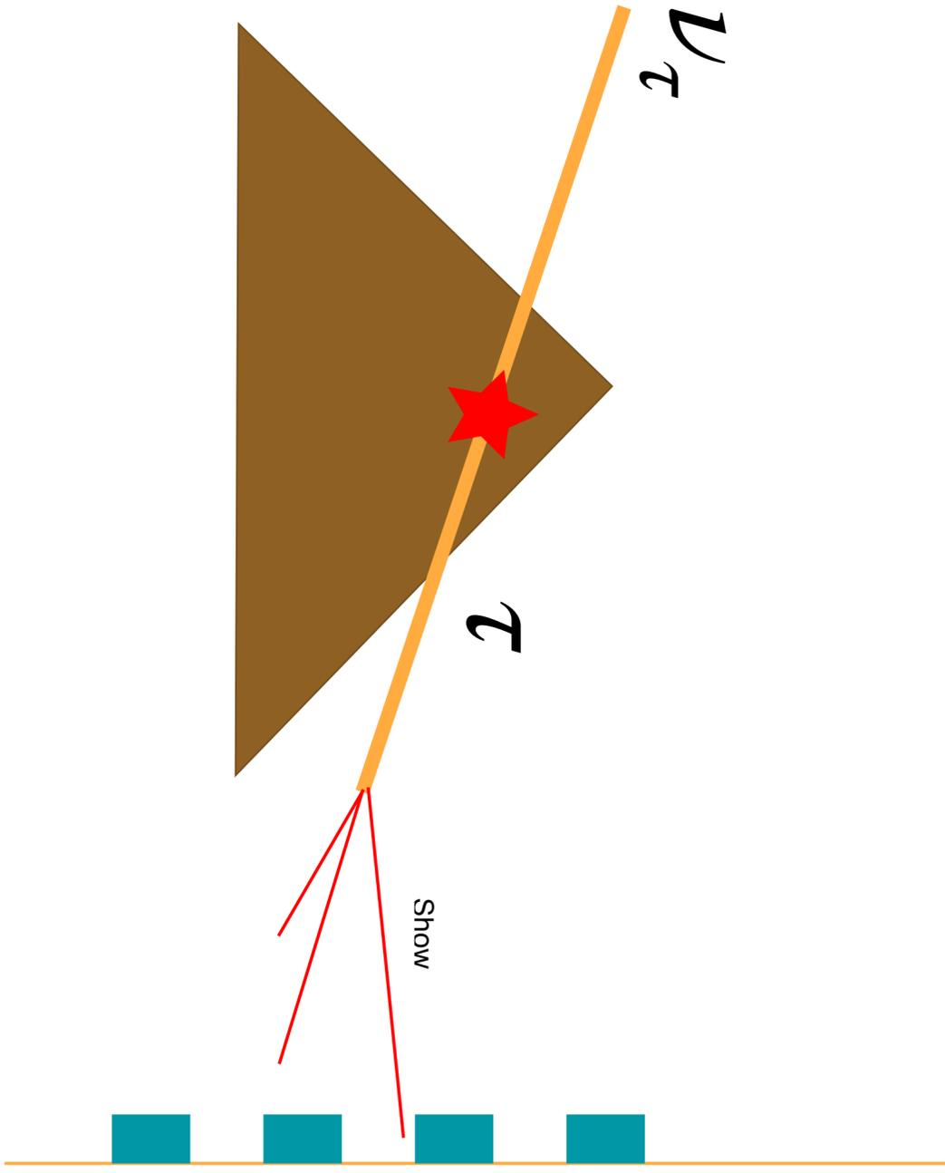
The geometry here is key for the acceptance of neutrino detection
