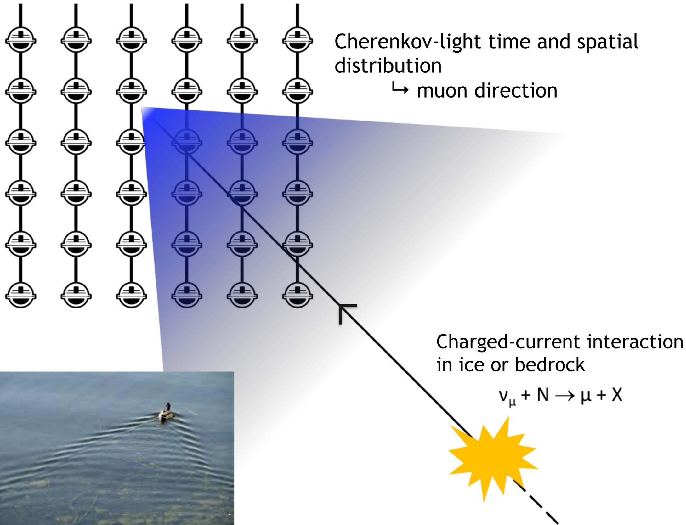
Principle detection mechanism of neutrino telescopes is Cherenkov light.
