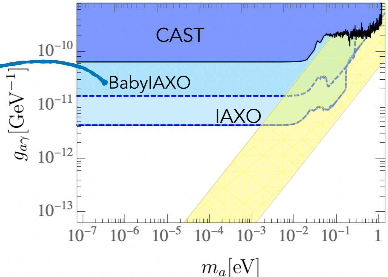
$$P_{a\gamma} = \left( \frac{g_{a\gamma} BL}{2} \right)^2 \frac{\sin^2(qL/2)}{(qL/2)^2}, \quad \text{with} \quad q \simeq \frac{m_a^2 - m_\gamma^2}{2\omega}$$
