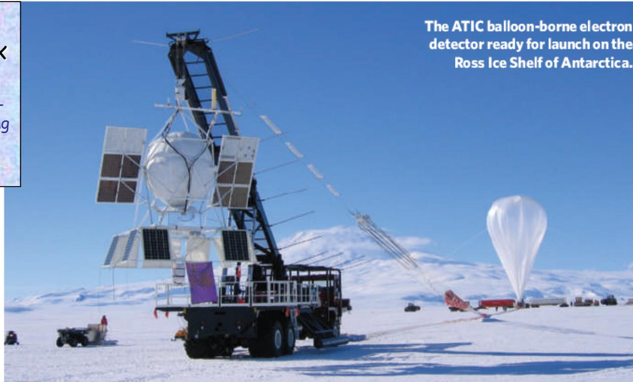
The ATIC balloon-borne electron detector ready for launch on the Ross Ice Shelf of Antarctica.
