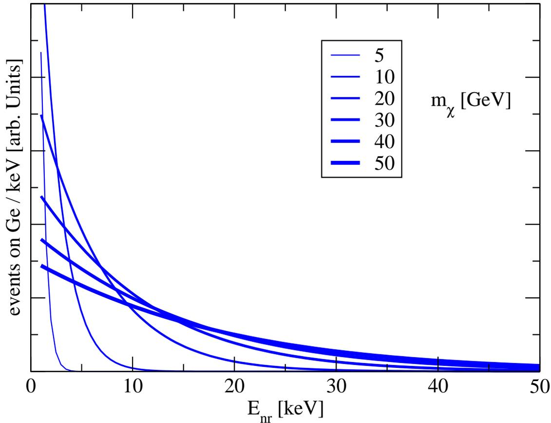
spectrum gets shifted to low energies for low WIMP masses  $\Rightarrow$  energy threshold is crucial
