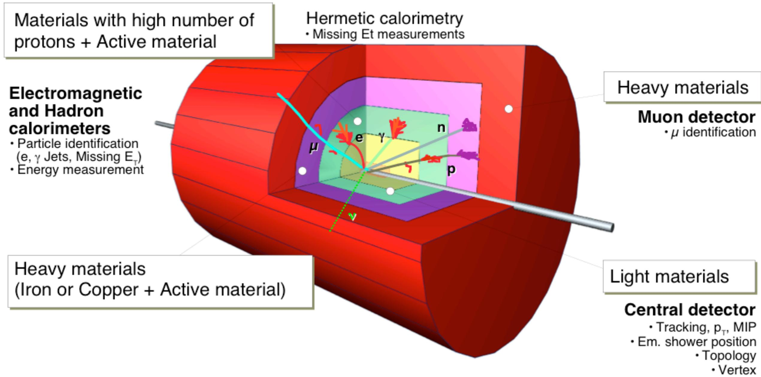
**Each layer identifies and enables the measurement of the momentum or energy of the particles produced in a collision**
