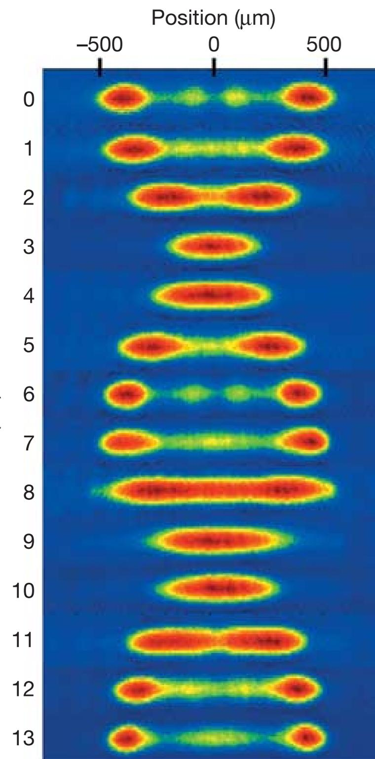
Here we report the preparation of out-of-equilibrium arrays of trapped one-dimensional (1D) Bose gases, each containing from 40 to 250  $^{87}\text{Rb}$  atoms, which do not noticeably equilibrate even after thousands of collisions. Our results are probably explainable by the well-known fact that a homogeneous 1D Bose gas with point-like collisional interactions is integrable.
