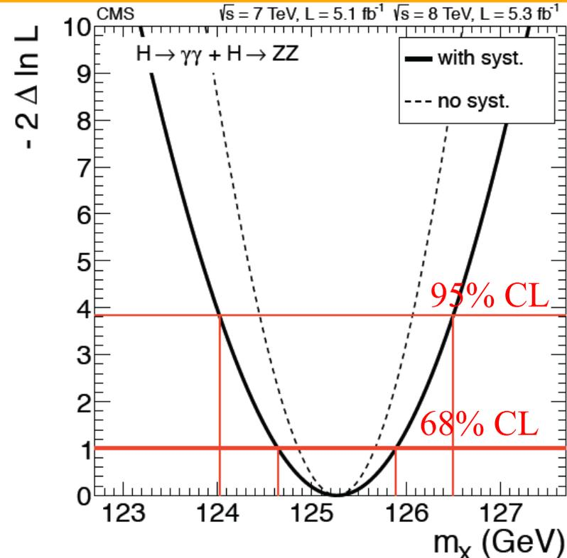
Model independent  $M_X$  scan with independent cross section but constraint of a unique mass
