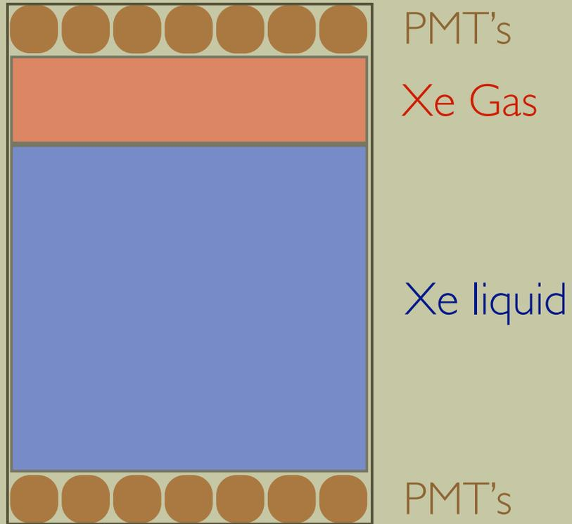
two-phase xenon time projection chamber
