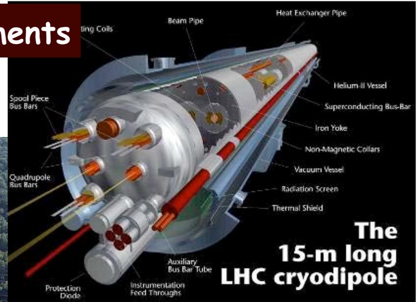
836 out of 1232 superconducting dipoles ( $B=8.3$  T) produced as of last Friday
