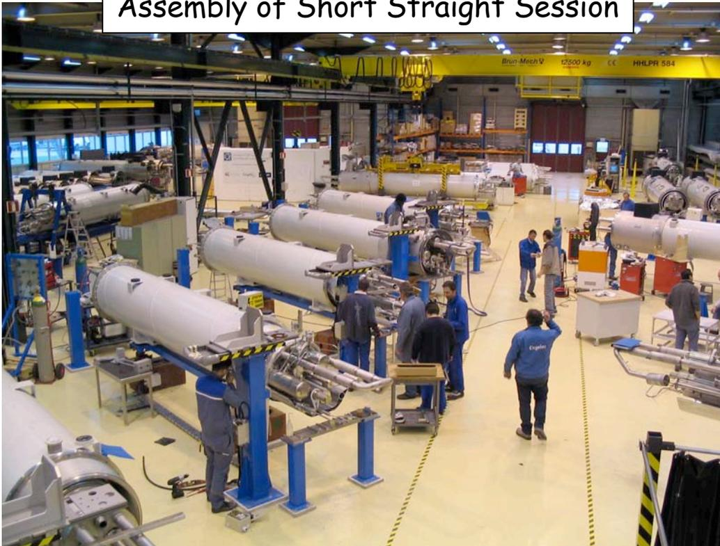
Inner triplet quads assembly
