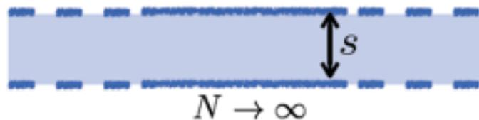
$$\mathcal{F} = \underbrace{\frac{s \rightarrow \infty}{s N} \text{ volume} \times f_b + \frac{2 N}{N} \text{ surface} \times f_s}_{N f_{ex}(s)} + \underbrace{\text{finite-size corr. } (s)}_{f_{ex}(s) \xrightarrow{s \rightarrow \infty} 2 f_s} \propto N$$
