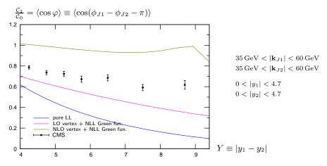
The NLO corrections to the jet vertex lead to a large increase of the correlation
