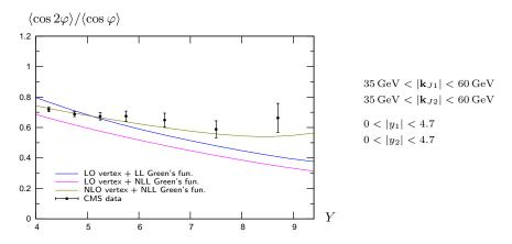
It is necessary to include the NLO corrections to the jet vertex to reproduce the behavior of the data at large  ${\cal Y}$
