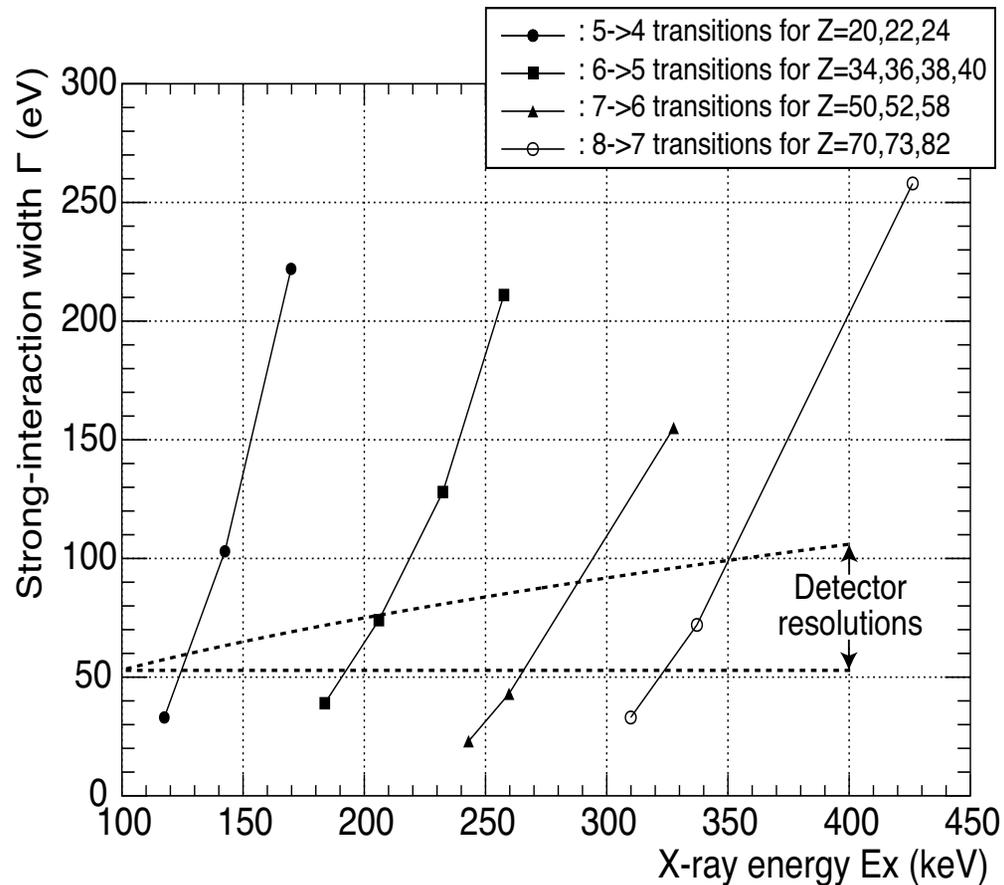
For these targets, both upper-level and lower-level can be studied simultaneously owing to a  $\approx 50$  eV resolution of new microcalorimeter detectors.
