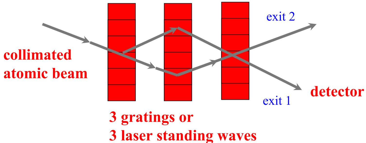
The mirrors and beam-splitters of the Mach-Zehnder optical interferometers are replaced by **elastic** diffraction on gratings. In the Bragg regime, diffraction of order  $p$  can be used.
