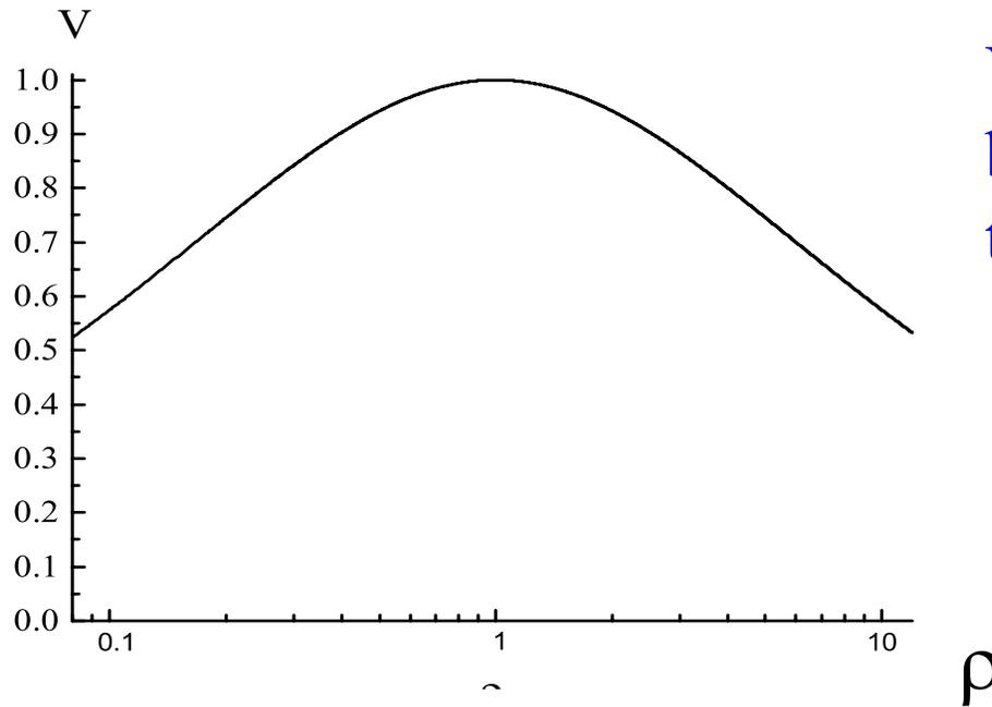
Visibility  $V$  as a function of the beam intensity ratio  $\rho$  for two-beam interference fringes.
